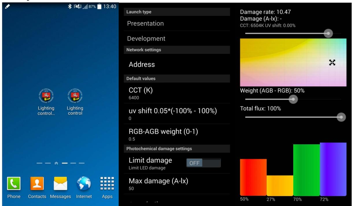
3. Plug the power supply to the Lume-20R luminaire and turn on Bluetooth connection on your android device. For the first time, pair the luminaire with your device using pairing code **1234**.
